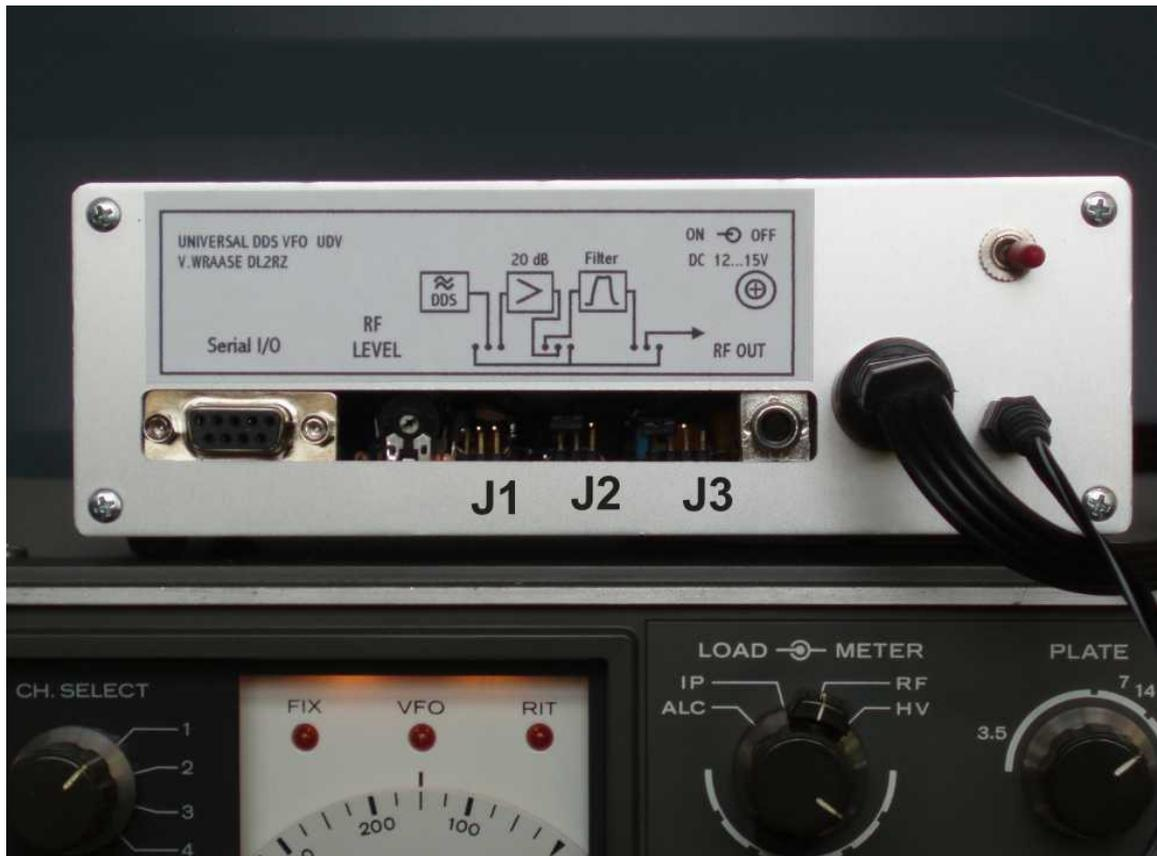
In the configuration "amplifier + Band pass Filter" You are always on the safe side, but should set the output level as low as possible. The best way to find the right value is to turn the transceiver on (tune) and carefully increase the level until the saturation (maximum transmitting power) is just being reached.
