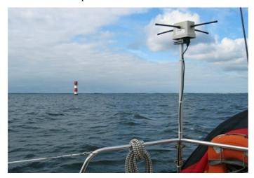
Reception often is degraded by broadband interference noise radiated from all kind of electronic devices, ranging from computers, tv-sets to coffee machines and all kind of switching power supplies. Keep the antenna several meters away from such possible noise sources. If in doubt disconnect these device(s) from power and check if satellite reception is improved. The level indication on the APT-06 receiver may help to analyse interfering noise levels.
