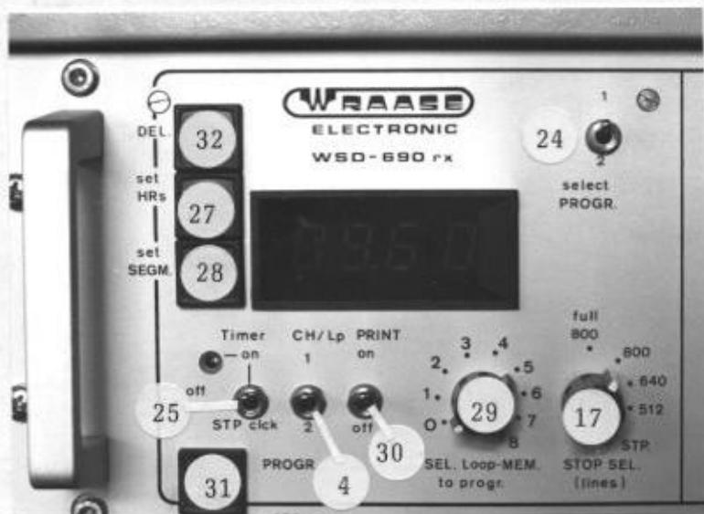
Fig.9: Programmable Timer Controls
